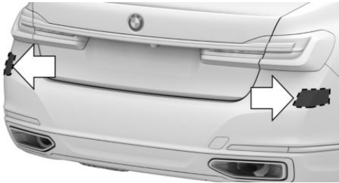
The radar sensors are located in the rear bumper.
