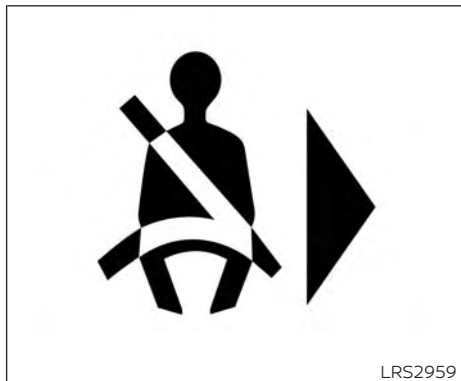
Passenger's seat belt warning light
