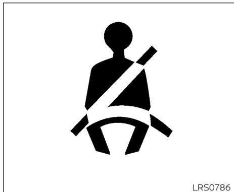
Driver's seat belt warning light
