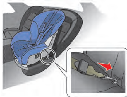
Forward-facing web-mounted — step 2
