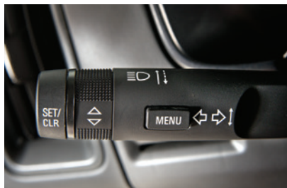
Base DIC Controls
