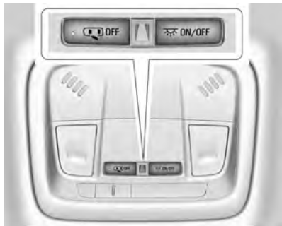
Dome Lamp Controls
