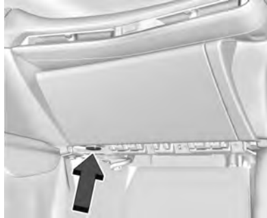
Interior Power Outlet
