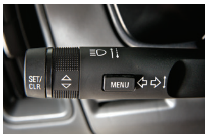
Base DIC Controls
