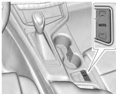
Driver Mode Control Switch
