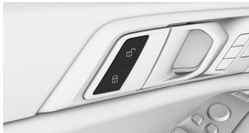
Buttons for the central locking system.
