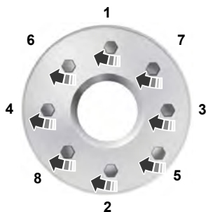
8-lug nut torque sequence
