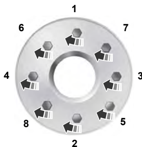
8-lug nut torque sequence
