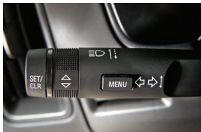
Base DIC Controls
