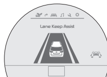
When the LKAS sensor detects the lane traveling in, both lanes are illuminated
