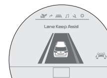
When the LKAS sensor detects the vehicle veering outside of the lane traveling in, a vehicle crossing lane indicator will illuminate, either on the left or right lane (shown in both images above)
