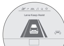
When the LKAS sensor detects the vehicle veering outside of the lane traveling in, a vehicle crossing lane indicator will illuminate, either on the left or right lane (shown in both images above)
