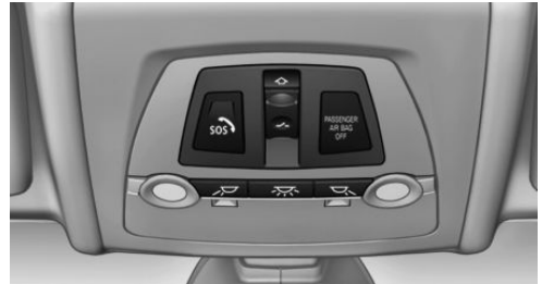
SOS button in the roofliner
