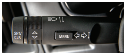
Base DIC Controls
