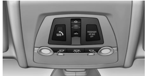
SOS button in the roofliner
