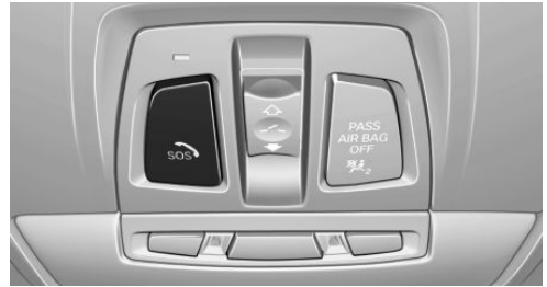
SOS button in the roofliner
