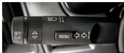
Base DIC Controls
