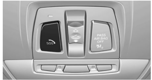
SOS button in the roofliner
