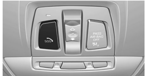
SOS button in the roofliner
