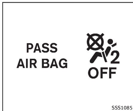
Front passenger air bag status light
