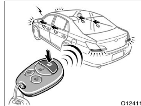
Locking operation (vehicles with key cylinder-type ignition switch)
